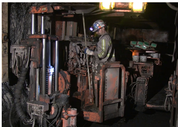
Fig. 5 A human operator is installing a bolt into the roof bolter ( https://bit.ly/3tfYOMY )
