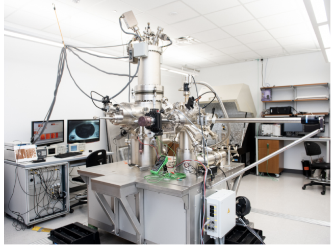
Fig. 2. Shows an STM. The left panel, borrowed from Wikipedia, shows the schematic of an STM. The right panel, borrowed from https://tmi.utexas.edu/facilities/instrumentation/scanning-tunneling-microscopes , shows an actual STM.
