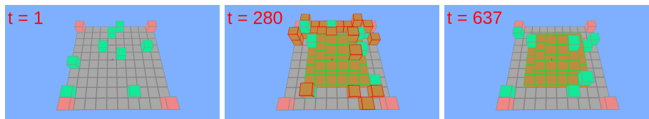
Fig. 7. Example frames of the construction of test structure 3 (Fig. 4), by a team of 8 agents (and respective time steps). Green-/red-edged cubes are correct/incorrect blocks, and solid green/pink cubes are agents/sources.
