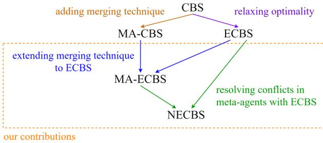
Figure 2: Relationships between CBS-related MAPF solvers. Arrows in the same color correspond to the same improvements. Our contributions include extending the merging technique from CBS to ECBS, resulting in Meta-Agent ECBS (MA-ECBS) and using ECBS to resolve the collisions between agents within the same meta-agent, resulting in Nested ECBS (NECBS).
