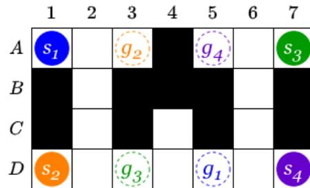
Figure 1: An illustrative 4-agent MAPF instance. Each start vertex  $s_i$  of agent  $a_i$  is shown as a solid circle, while its goal vertex  $g_i$  is shown as a hollow circle in the same color.
