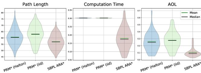
Fig. 9. Path length, computation time and AOL for different sampling strategies, namely PRM\* using deterministic Halton sampling (left), PRM\* using random uniform sampling (center) and the lattice-based motion-planning algorithm ARA\* (right). All performance metrics are reported with a computation time limit of 0.3 seconds each (to be fair to the fast ARA\*) in 100 random indoor-like grid-based environments with a desired minimum corridor width of 3 cells.
