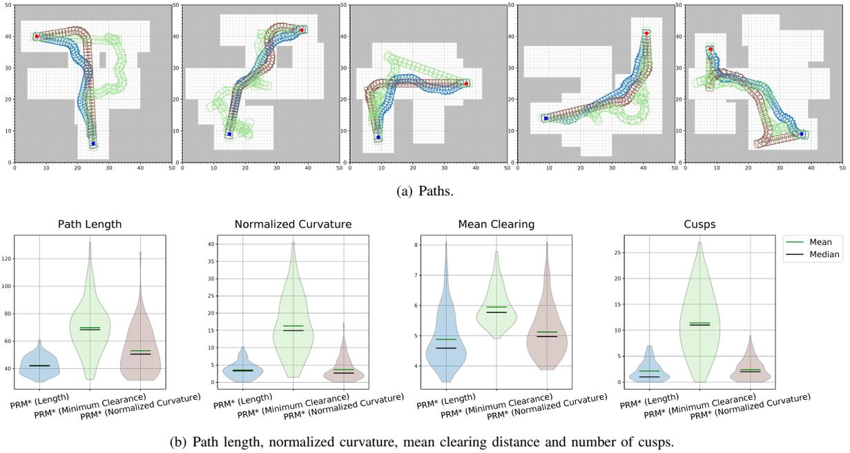
Fig. 10. Results for different optimization criteria, namely PRM\* with minimizing path length (left), maximizing minimum clearing distance (center) and minimizing normalized curvature (right). The colors of the paths (top) correspond to the colors of the optimization criteria (bottom). All metrics have been computed with a time limit of 2 seconds each in 100 random indoor-like grid-based environments with a desired minimum corridor width of 5 cells.
