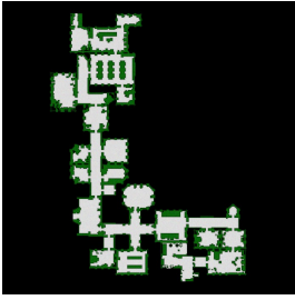
(a) State lattice has 68,208 vertices and 135,310 edges.
