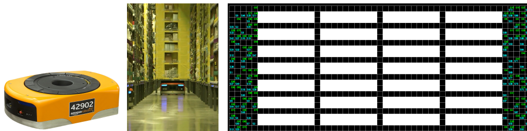
Figure 1: Warehouse robot (left), inventory pods (center), and the layout of a small simulated warehouse (right). The left and center photos are courtesy of Amazon Robotics.
