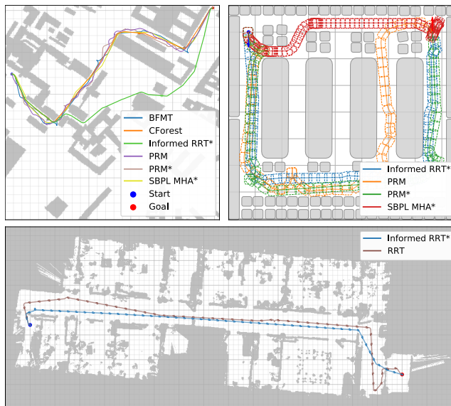
Figure 1: Selection of environments provided by Bench-MR: City grid from the Moving AI path-finding benchmark (Sturtevant 2012) (top left), polygon-based warehouse environment (top right), and thresholded occupancy grid from the Freiburg SLAM dataset (Kümmerle et al. 2009) (bottom).
