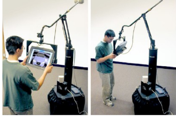
Figure 6: The Boom Chameleon interface. As the user moves the monitor around, the image on the display updates as if the user were moving a picture frame around a physical object (Tsan02).
