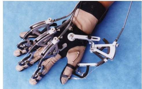
Figure 2: The Immersion CyberGrasp glove. This is an example of a haptic device which uses the body as its anchor (Glas07).
