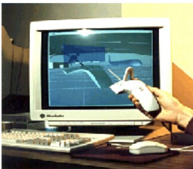
Figure 5: The Virtual Tricorder. The top portion shows it in the virtual realm with context dependent information displayed. The lower portion shows the physical object and its virtual counterpart.
