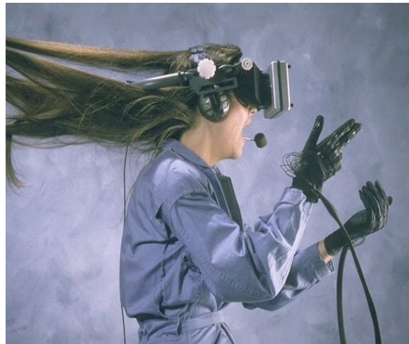
Figure 1: An image showing the state of the art in virtual reality, from 1989. Note the lack of physical feedback for the user (Carl06). Originally presented in (Fish89).
