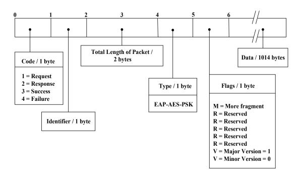
Figure 3-3: EAP-AES-PSK Packet Format
