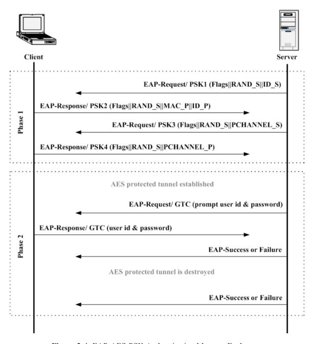
Figure 3-4: EAP-AES-PSK Authentication Message Exchanges
