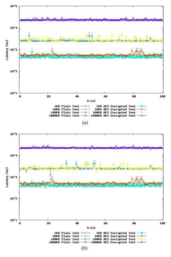
**Figure 4-3**: (a) Server Completion Time in the Un-Controlled Environment, (b) Client Completion Time in the Un-Controlled Environment
