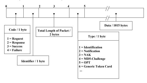
Figure 2-4: EAP Packet Format [2]
