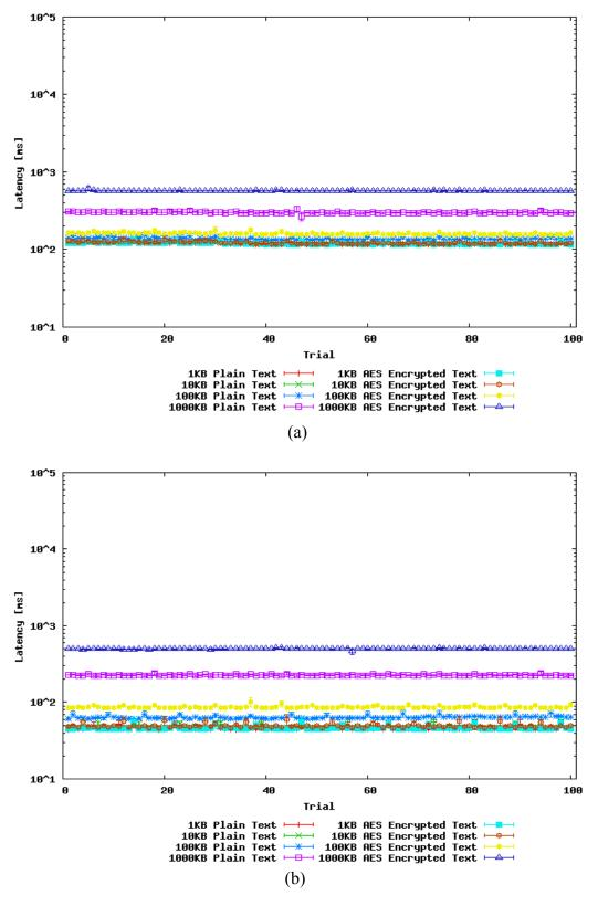
**Figure 4-2**: (a) Server Completion Time in the Controlled Environment, (b) Client Completion Time in the Controlled Environment
