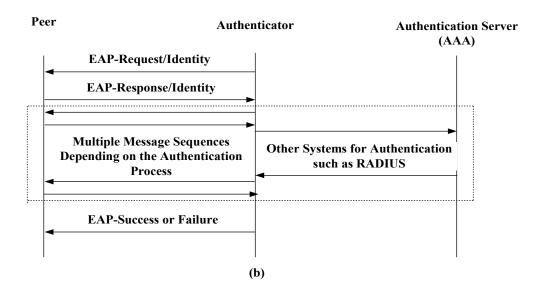
**Figure 2-3:** (a) EAP Message Exchange without AAA, (b) EAP Message Exchange
